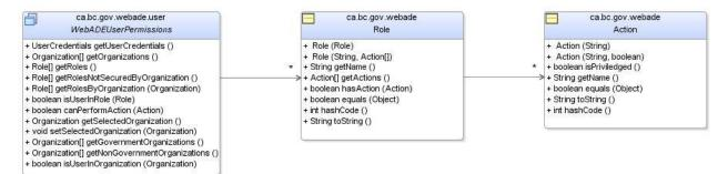
WebADE uses these authorizations to restrict user access at two points: 1) At the point of request, before a business code is executed and 2) At any time that access is required to the application's database.
