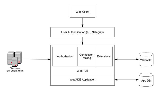
The WebADE is comprised of several components. From a developer's point of view, there are two main pieces, a set of Java libraries and a supporting database table structure.
