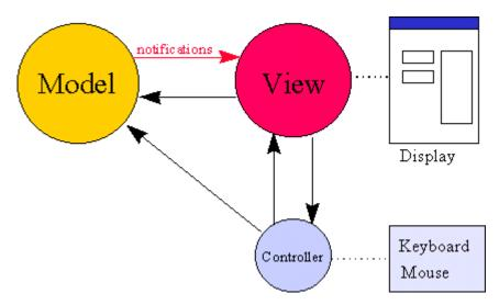
The current suggested framework for MVC for WebADE is Apache Struts, which is described below. Regardless of which framework is used, the main concept of MVC, as it pertains to web applications is that of using a controlling Servlet to handle all requests to a web application. This means that every link and form in web pages that are part of the "View" section of the application will send a request to the "Control" Servlet that controls the web application.
